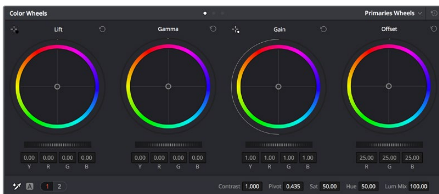
The 'lift', 'gamma', 'gain' and 'offset' color wheels give you total control over the color and tonal balance of your clips. To make a uniform adjustment to all colors for each tonal region, drag the dial underneath the color wheels back and forth
